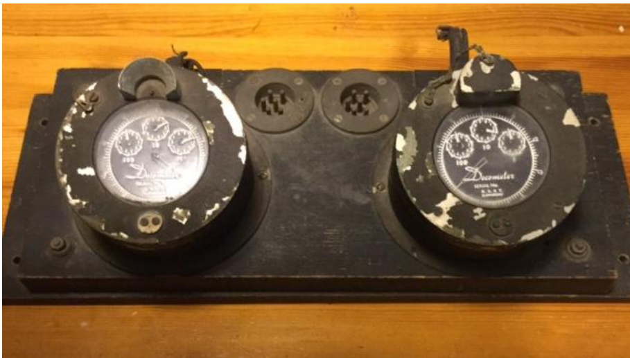
The set of dials now part of the Medusa collection; these were originally made from modified gas meters.
