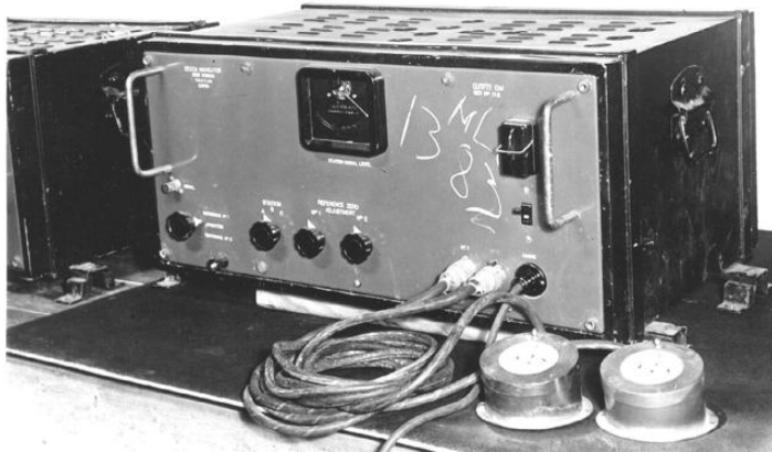
QM equipment from ML1383, the other Omaha vessel, showing the dials on extension leads.
